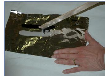
Spread a sheet of aluminum foil and mix the epoxy resin and hardener in the recommended proportions. Evenly spread a thin layer of mixed adhesive completely over the surface of one of
