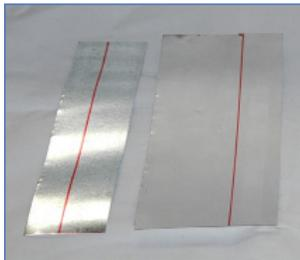
Mark cut lines with a marker and carefully cut with a pair of tin snips, available from a hardware store.
