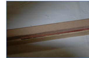
Allow the adhesive to cure according to the manufacturer's directions (usually overnight).
