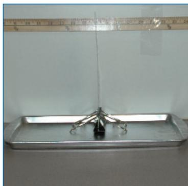
Slowly heat the strip with a hair dryer, keeping the dryer at a fixed distance from the strip. Point the dryer at the thin side of the strip so that it does not move.
